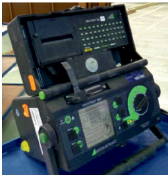
Test of electrical continuity
